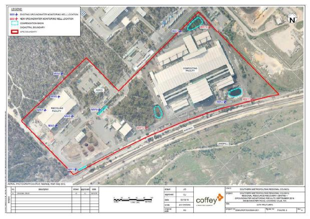
Figure 5: Map showing the stormwater retention basins within Part Lot 77 and Part Lot 78 on Plan 2903 Bannister Road Canning Vale WA 6155
